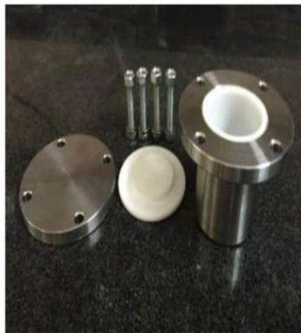
Figure.1.8 Steel autoclave with Teflon liners
