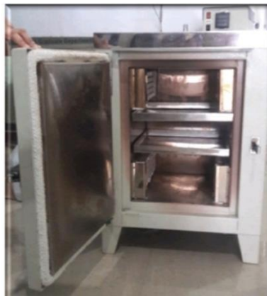
Figure.1.9 Hydrothermal oven used for synthesis
