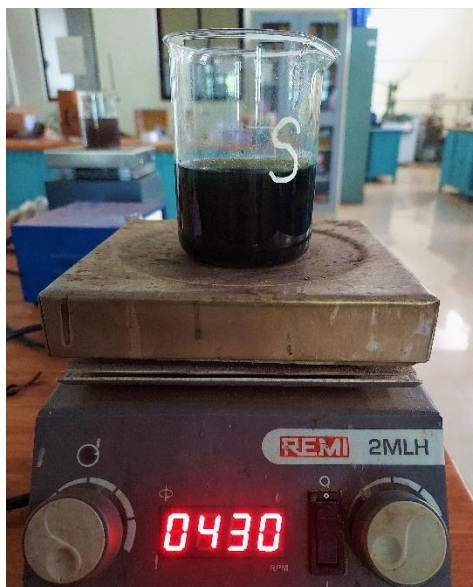
Fig 9: Preparation of ALG-chitosan- H. colorata polymer by solvent casting process.
