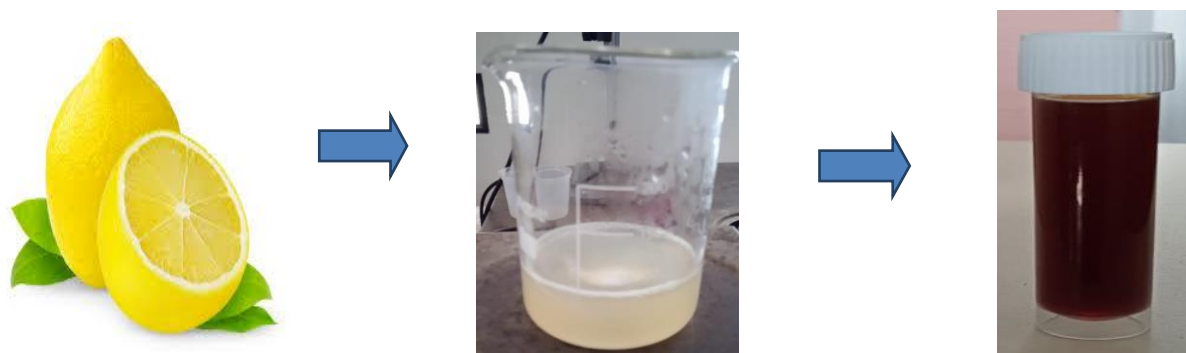
Figure 4.1 : Schematic representation of synthesis of carbon dots from lemon juice.
