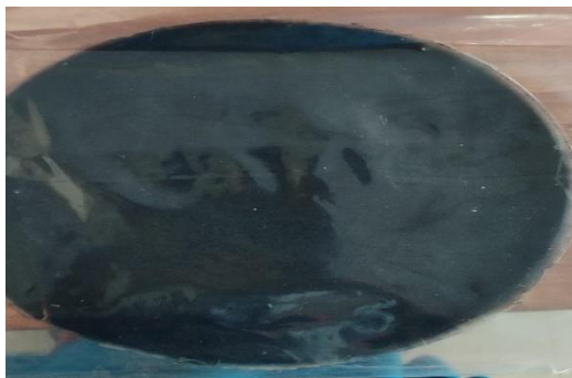
Fig 13. ALG-Honey-Charcoal-Citric acid-CaCl 2 film
