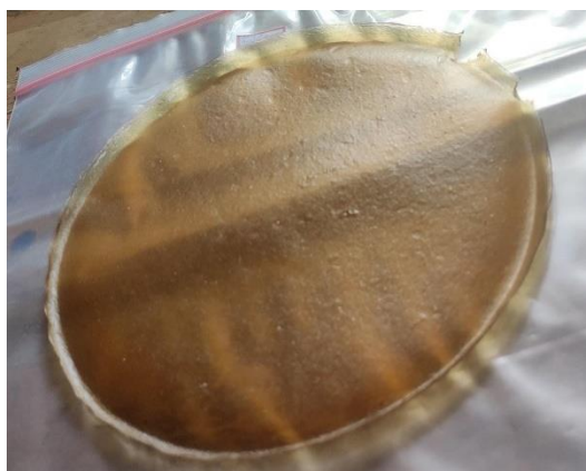
Fig 10. ALG-Honey-Citric acid-CaCl 2 Film
