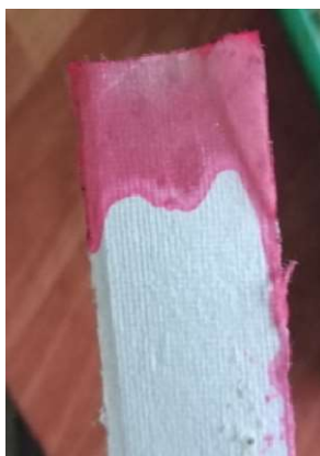
Figure 6. Spot test for Furfural
