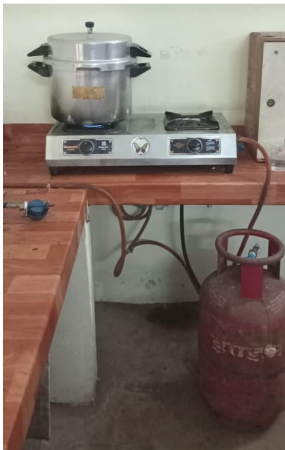
Figure 4: Experimental setup for hydrothermal production of Furfural
