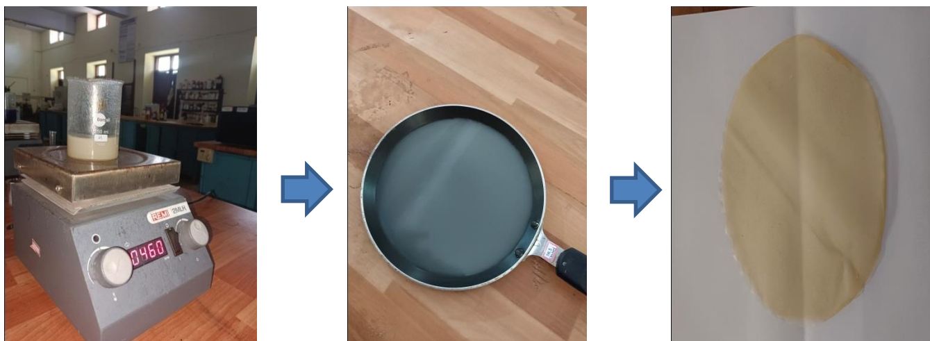
Figure.5 Fabrication of CD-AgNP/CNW- SPI polymer films for packaging
