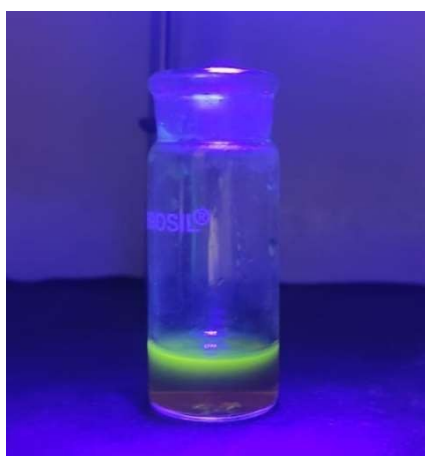
Fig: Solution of carbon dots under UV lamp
