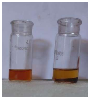
Fig: carbon dots in NaOH solution (left) and HCl solution (right)
