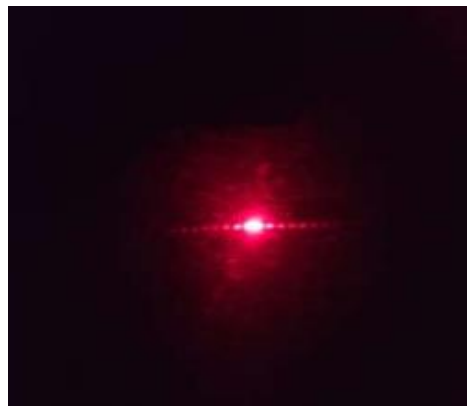
Fig 3.1 Slit obtained by using single slit
