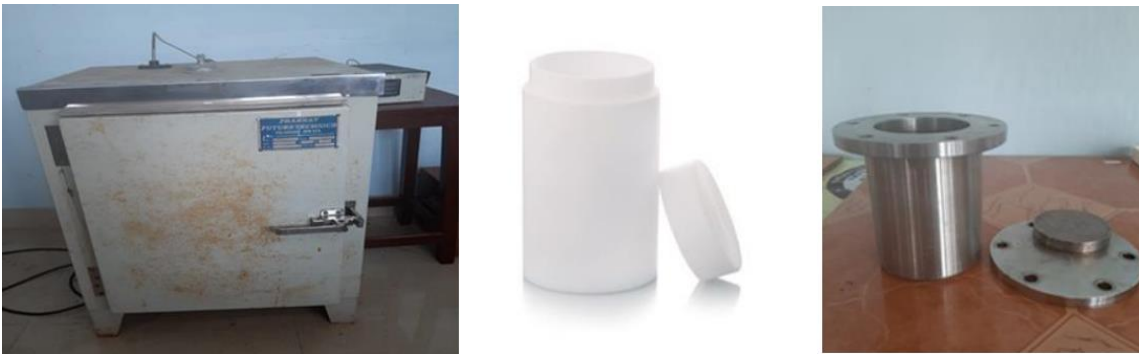
Fig 1.15: The hydrothermal reaction set up and the Teflon jar and the stainless-steel autoclave with screws
