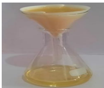
Figure 2.5 Filtration after the formation of CeO 2 nanoparticles.
